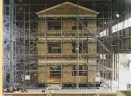
Lateral loading test on the wooden house
