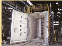
Fire resistance test
